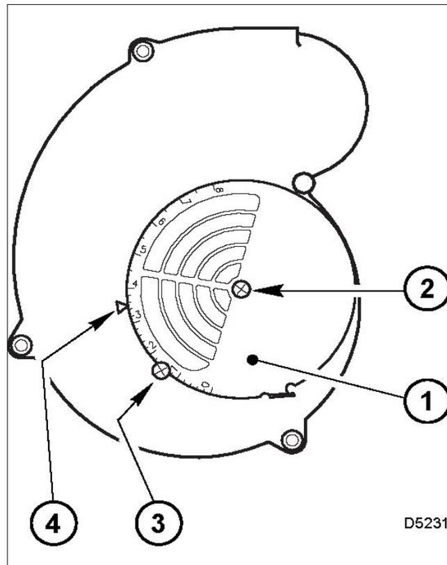
**B)** The proper number on the manual AIR ADJUSTMENT PLATE (1) should line up with the SETTING INDICATOR (4) on the fan housing cover. Once set, the air adjustment plate should be secured in place by tightening SCREWS 2 and 3.
